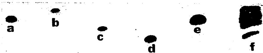
Fig. 4. TLC separation of five barbiturates. a = Pentobarbital; b = secobarbital; c = phenobarbital; d = butobarbital; e = amobarbital; f = mixture of a, b, c, and e. Solvent, chloroform-acetone (88:12).
